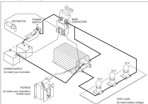
Fig. 20 Setup for bench testing.
