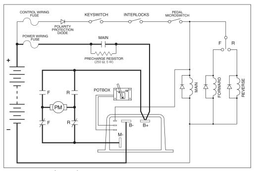
Fig. 15 Basic wiring for use with PM motors.
