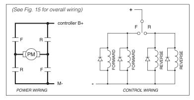
A better approach — and the one we recommend — is shown in Figure 17. The motor is reversed by the two single-pole, double-throw (2×SPDT) contactors. A third contactor (SPST) opens the motor circuit in neutral or when the pedal is released, allowing the motor to freewheel.
