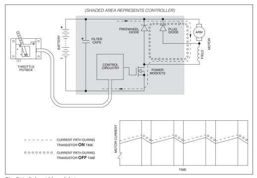
Fig. B-1 Pulse width modulation.
