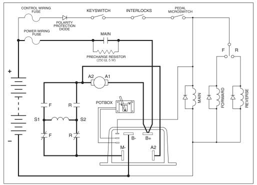
**Fig. 6** Basic wiring configuration, Curtis 1204/1205 controller.
