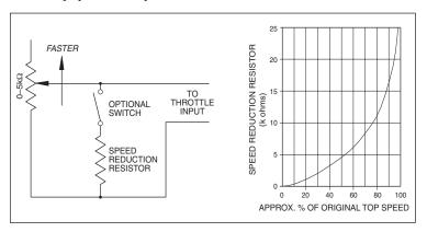
load. You should determine by experiment the proper resistor value to give the desired speed reduction. (NOTE: with reduced speed operation, only top <u>speed</u> is reduced; full <u>power</u> is maintained for starting at low speeds.)
