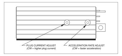
Use the following adjustment procedure. The keyswitch should be off during adjustment.
