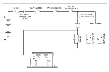
contacts is added on the forward/reverse switch. Therefore, a double-pole, double-throw (DPDT) center-off switch must be used for this setup. A "hesitation switch" is recommended, to ensure the switch is in neutral long enough to actuate HPD and inhibit plug braking.
