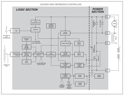
Fig. A-1 Block diagram, Curtis 1204/1205 controllers.
