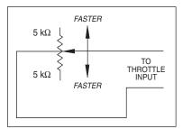
of which direction the twist grip is turned. Alternately, a 4-terminal, center-tapped 10 k $\Omega$  pot can be coupled directly to the twist grip, as shown in Figure 11.
