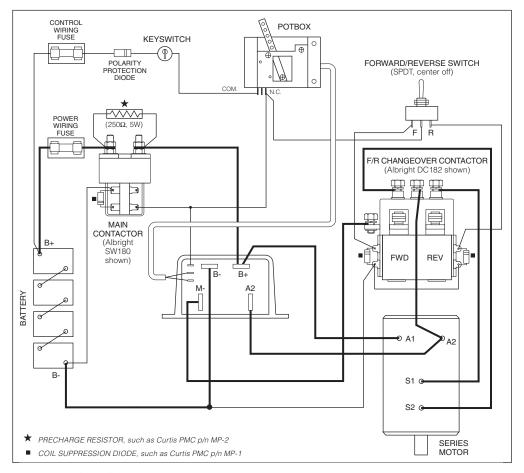
Fig. 5 Typical installation, Curtis 1204/1205 controller.
