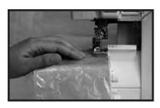
Set up the machine for 2-thread flatlock - wide but the needle threading path is different for this technique.
