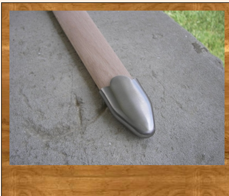
The chape end of the core. Notice the chape is a bit loose here.. so it will fit over the leather.
