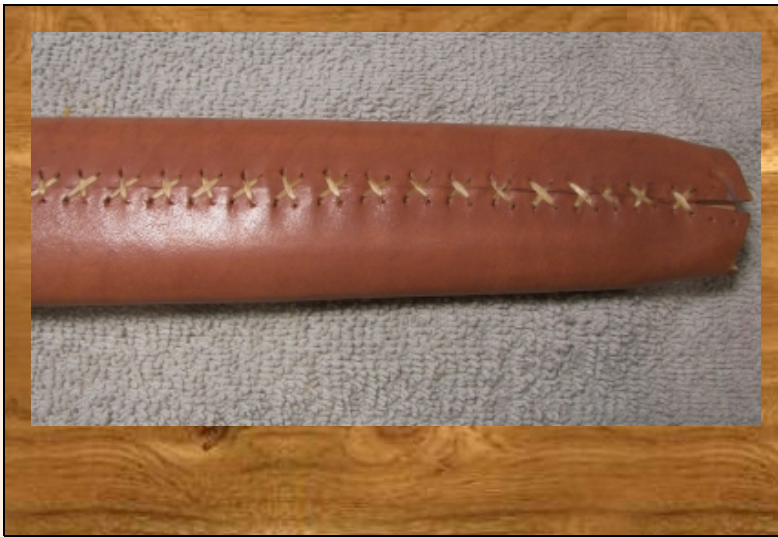
This shows the back of scabbard (wet leather) with the sewing completed.
