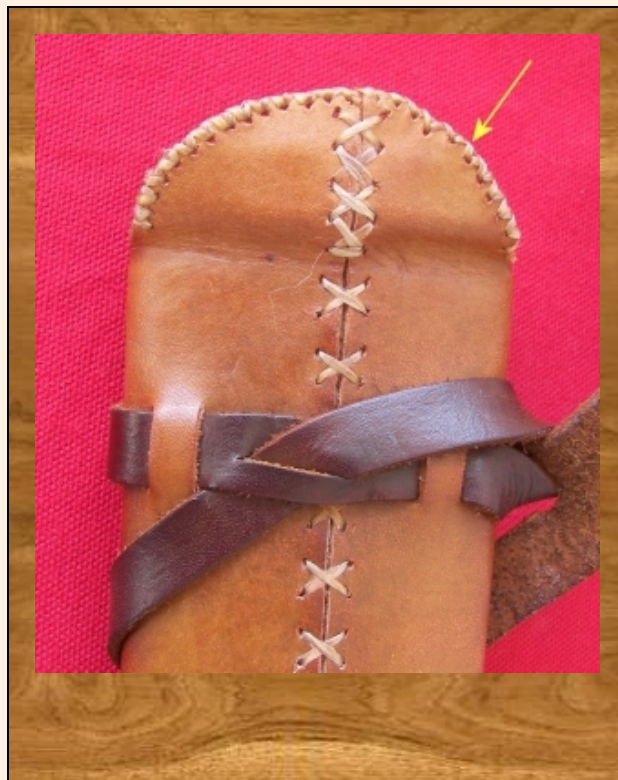
This shows the back of scabbard (wet leather) with the sewing completed.
