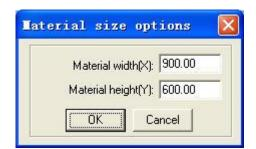
**Material width(X):** It is the width of the work piece (the default is the worktable's width).
